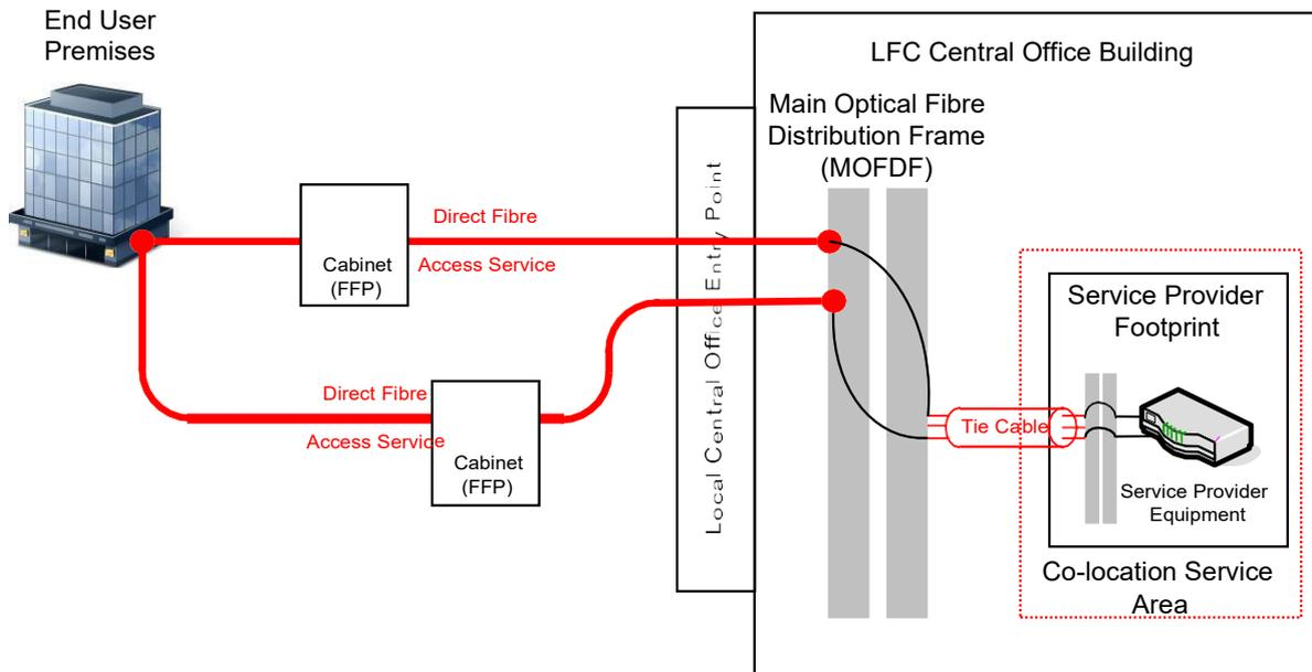
*Single Central Office redundancy with separate diverse fibre and diverse access to End User Premises*
