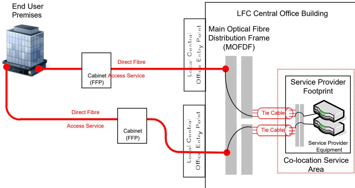
*Dual Central Office redundancy with separate diverse fibre, diverse access to End User Premises and diverse access to a separate Central Office*
